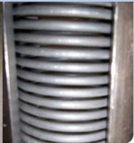
*"..., for a given length of well completion and unit pressure draw-down values, we may anticipate continuously wound wire spring screen technology should allow for substantial gains respecting the flow of reservoir fluids over that of slotted liner."*
